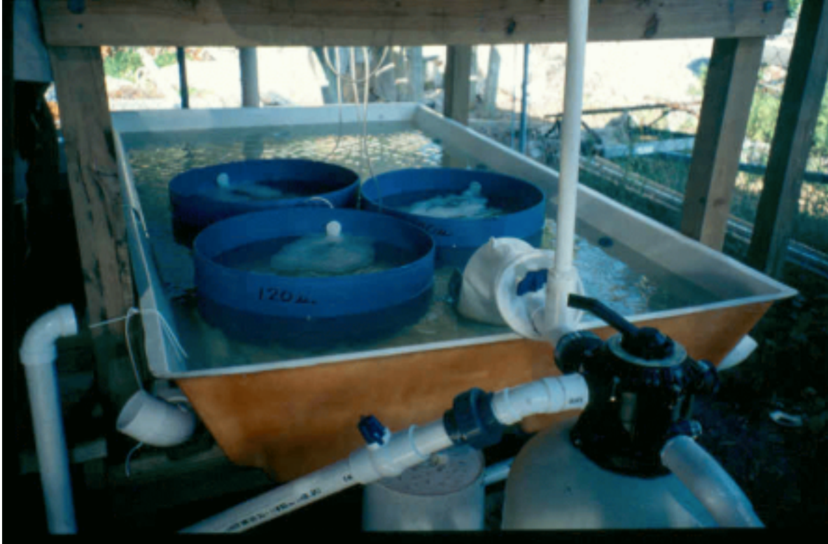
Figure 5. Remote setting unit including 250-gallon tank, sand and bag filtration, and 3 downwellers.
