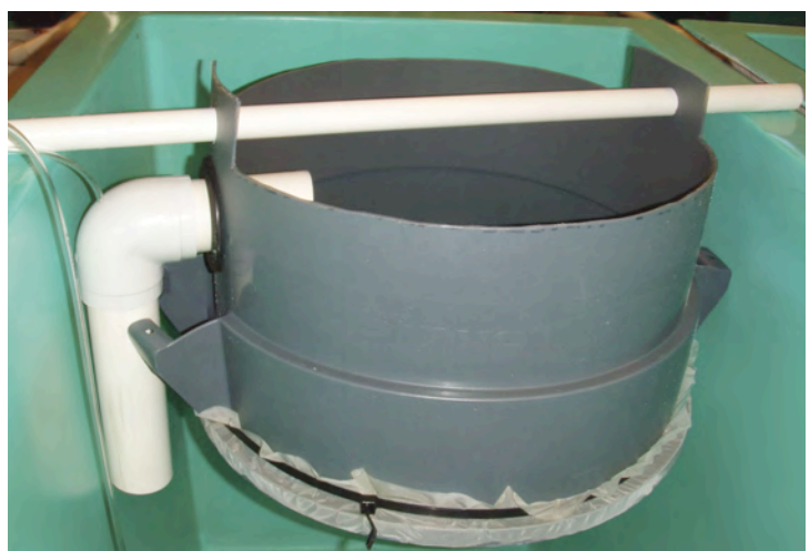
Figure 9a and b. Silos installed in fiberglass tanks are supplied with seawater by airlift pumps and used to hold larval clams during metamorphosis.
