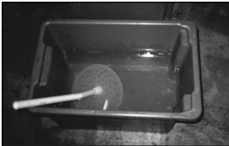
Figure 26. A “plunger” style egg mixer ensures an unbiased sample is taken by avoiding a circular stirring motion.
