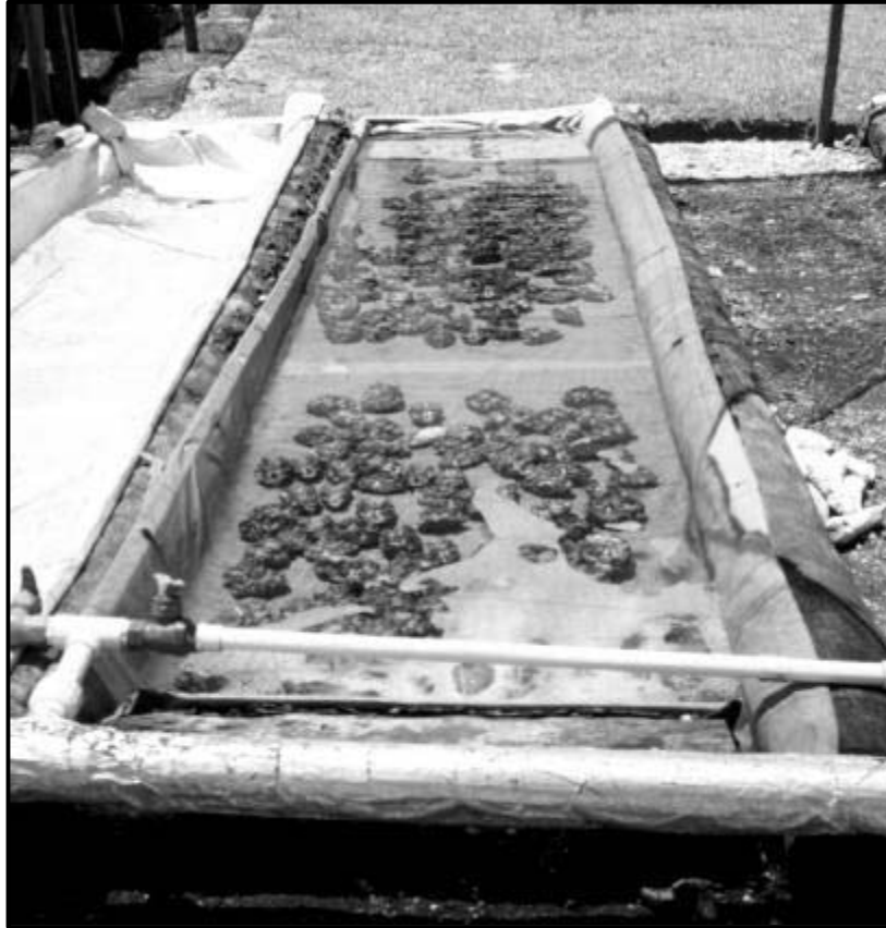
Figure 19. Holding tanks are constructed from coconut logs and vinyl liners at ICLARM's Coastal Aquaculture Center on Guadalcanal, Solomon Islands.
