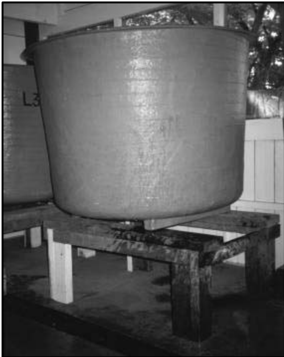
Figure 28. A locally made fiberglass larval rearing tank at ICLARM's Coastal Aquaculture Center on Guadalcanal in the Solomon Islands.
